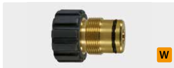
M27 AG : 3/8" IG. Messing *. Max. 400 bar
